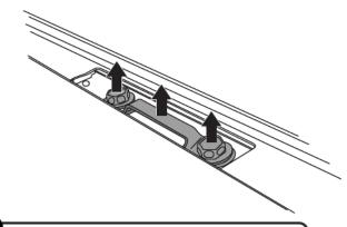
When loosening fasteners, keep switching between them to drop tension progressively. If not, the nutplate inside the roof cavity may come loose.
