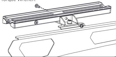
**NOTE -** The Pivot Mount assembly will still have movement after securing which is intended.
