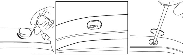
Note: Apply upwards pressure to the rail to prevent the captive nut from dropping and spinning while the bolt is being undone.
