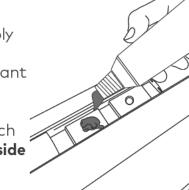
ASSEMBLE PIVOT BRACKET TO RUGGEDLINE
