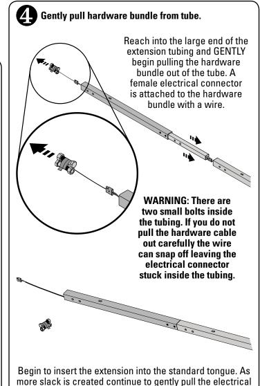
connector and wire out. Once the extension is completely inserted into the standard tongue, and the electrical connector has been fully exposed detach the wire from the
