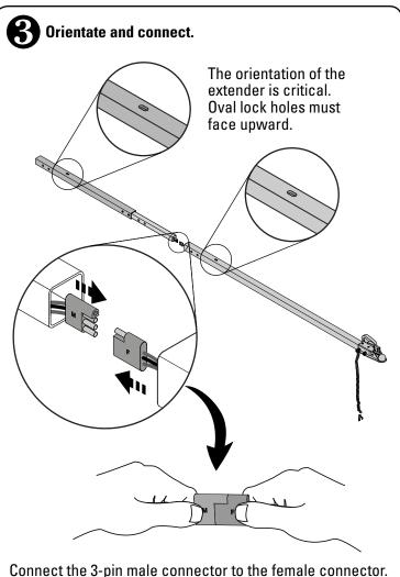
Be sure the connectors are firmly pressed together.
