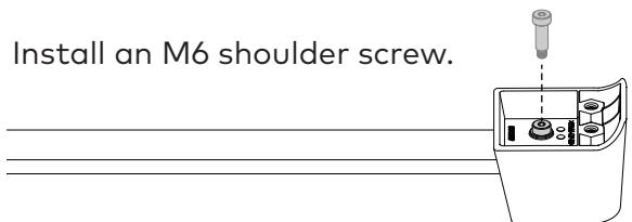
Using the provided wrench, tighten completely to 3 Nm.
