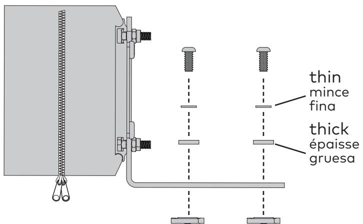
**NOTE:** The maximum unsupported distance from the bracket to the end of awning must not exceed 50" (127cm).
