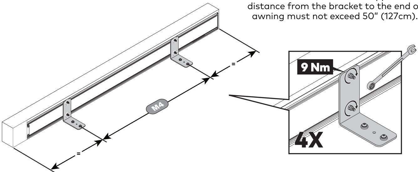
**NOTE:** It is recommended to make sure the pair of brackets are centered on the awning. Tighten completely to 9 Nm.
