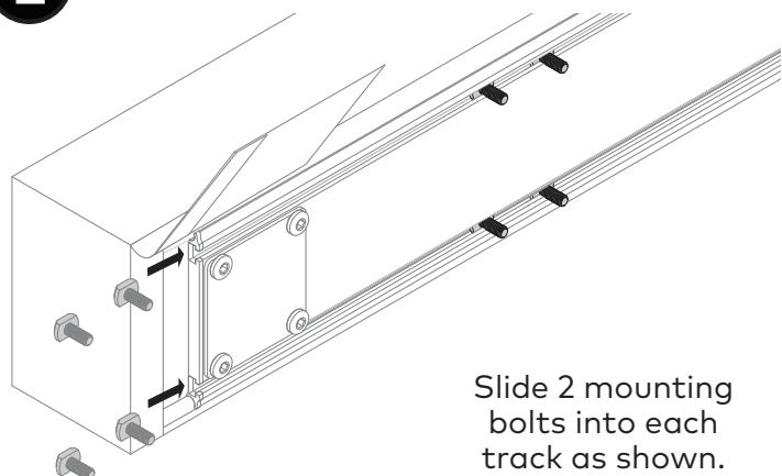
Slide 2 mounting bolts into each track as shown.
