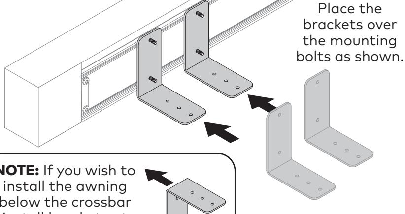
Place the brackets over the mounting bolts as shown.
