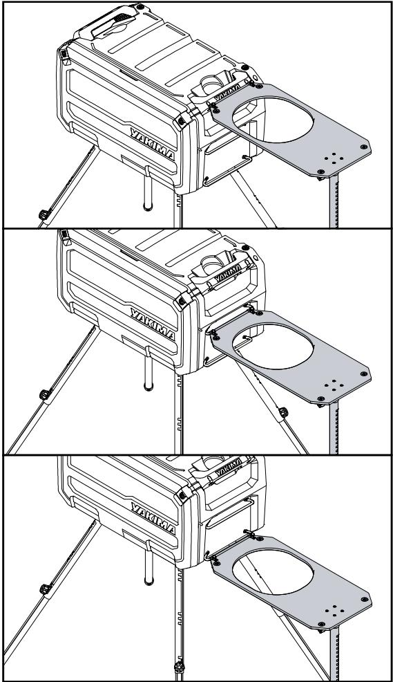
Remove the preinstalled retention screws from the hooks. Engage the hooks with OpenRange in your desired position and reinstall the retention screws.
