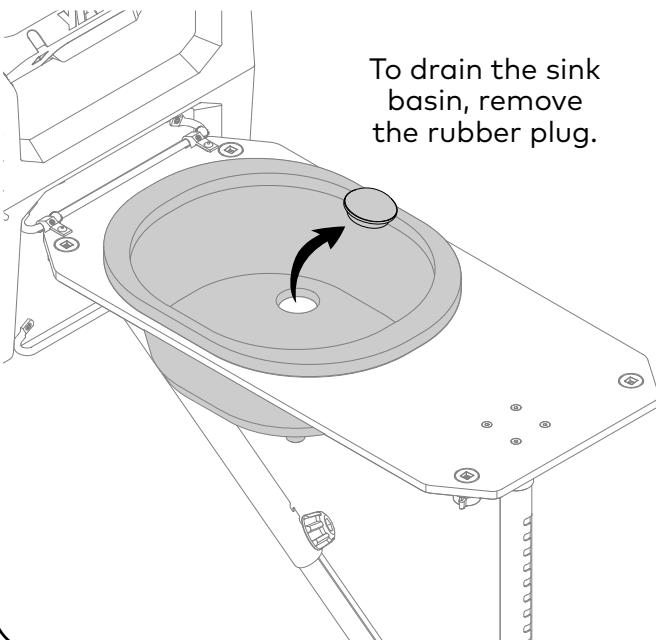
To drain the sink basin, remove the rubber plug.
