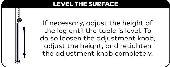
If necessary, adjust the height of the leg until the table is level. To do so loosen the adjustment knob, adjust the height, and retighten the adjustment knob completely.
