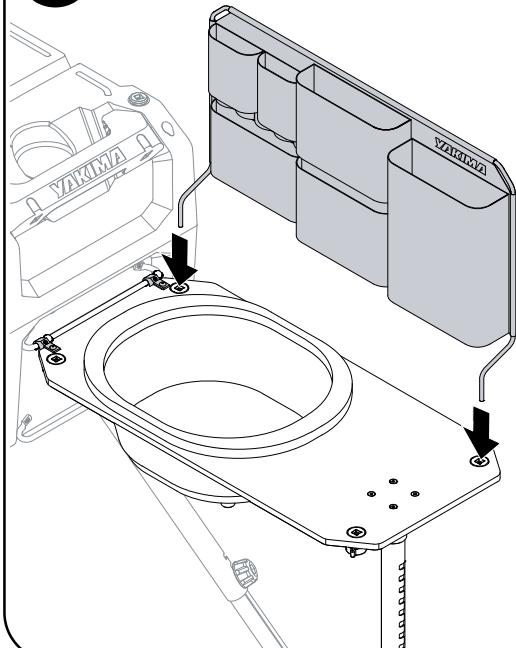
Install the backboard organizer by inserting it into the mounting points on the table.
