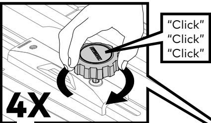
Use the torque wrench to fully tighten the clamps by slowly turning the wrench until it clicks 3 times. Visually inspect the clamps to make sure they are engaged with the crossbars. Stow the wrench in its storage spot behind the handle for easy access **NOTE:** The storage spot will loosen with use.
