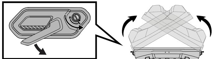
**NOTE:** The opposite side of the box must be fully closed (listen for a "click") with the key removed in order to open the other side.
