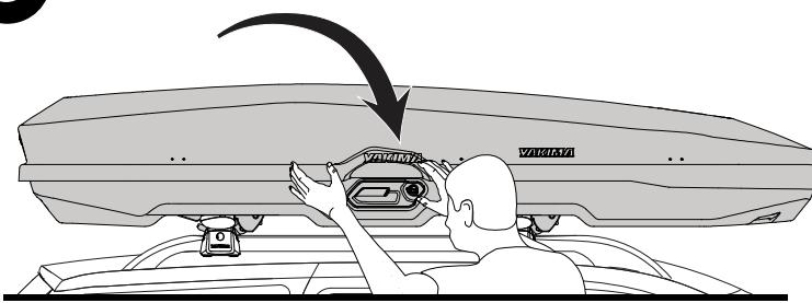
Push the lid down until the handle returns to a horizontal position and you hear a "click". The handle must return to the horizontal position to lock the box and remove key. Verify closure by pushing up on lid at both ends. **NOTE:** The key cannot be removed unless the lid is fully closed and locked.
