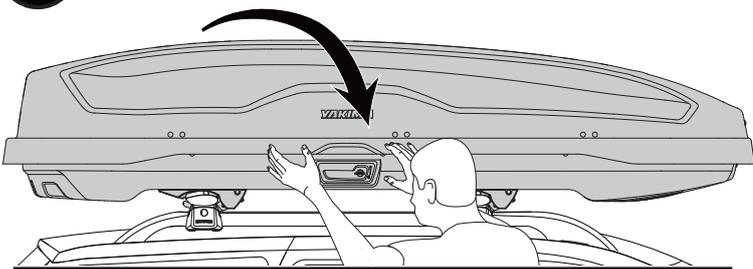
Push the lid down until the handle returns to a horizontal position and you hear a "click". The handle must return to the horizontal position to lock the box and remove key. Verify closure by pushing up on lid at both ends. **NOTE:** The key cannot be removed unless the lid is fully closed and locked.
