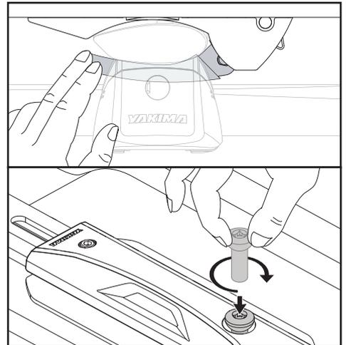
**NOTE:** If you accidentally remove the clamp nut, compress the clamp and thread the nut back onto the threaded post.
