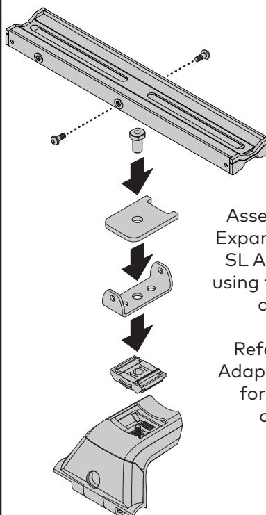
Assemble the LNL Expansion with your SL Adapter clamp using this illustration as a guide.
