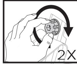
**Reinstall saddles.** Insert the saddles, slide them into position, and fully tighten them down.
