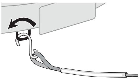
**15** Slide plastic tube to protect vehicle at contact point.
