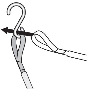
**14** Hook the strap to a metal surface on the bumper, tow loop, or frame hole using hook.
