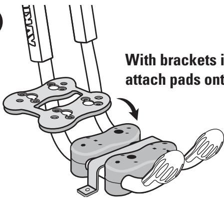
With brackets in place, attach pads onto bases.
