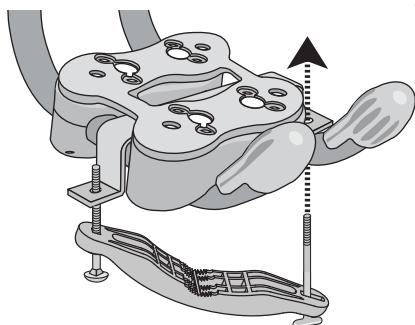
*Insert bolt into round hole, and T-bolt into slotted hole.*
