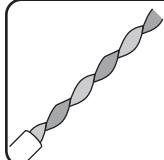
**NOTE:** Twisting the strap will help reduce wind vibration.
