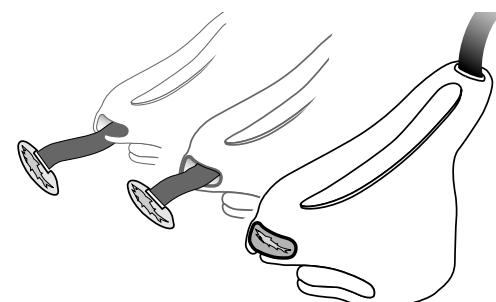
► Insert shark chucks securely into slot in nose of each saddle.
