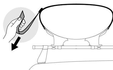
**Test movement by rocking boat.**
