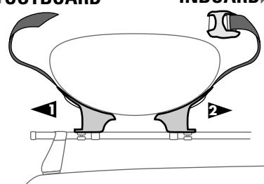
► Insert plain strap into notch at top of **OUTBOARD** saddle.
