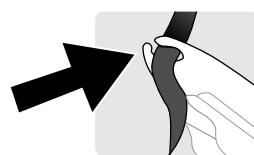
► Loop straps through saddle, placing straps in groove on underside of each pad.
