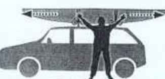
► BEFORE DRIVING AWAY: Tie down boat at front and rear. Tighten straps and hex keys.
