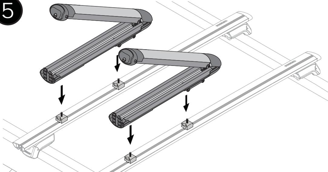
Place the mounts onto the blocks.
