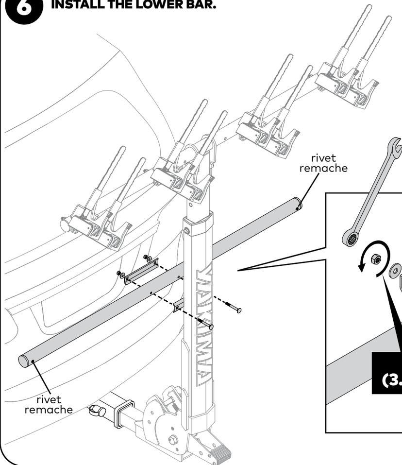
Use the 10 mm wrench to attach the lower bar to the mast with the carriage bolts, plate, washers, and nuts. Make sure that the rivets face outward as shown. Tighten to 5 Nm.
