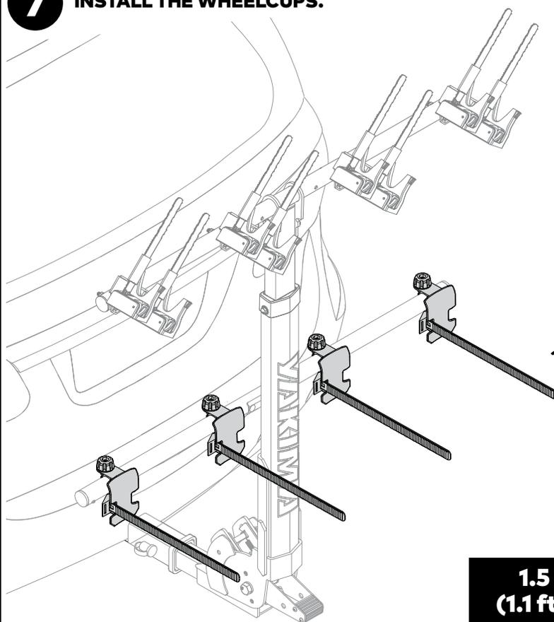
Loosen the knob and flex the wheelcup in order to clear the retention screw on the bar. Then rotate and space the cradles as shown. Tighten the knobs to 1.5 Nm once they are in position.
