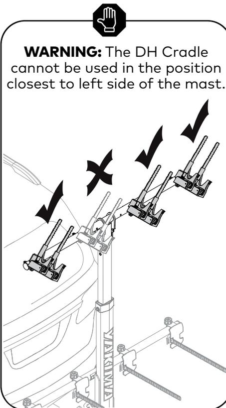
**WARNING:** The DH Cradle cannot be used in the position closest to left side of the mast.
