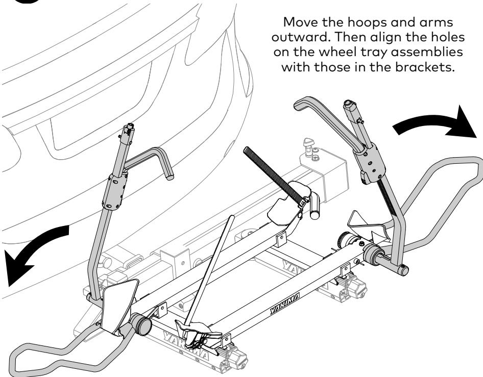
Move the hoops and arms outward. Then align the holes on the wheel tray assemblies with those in the brackets.
