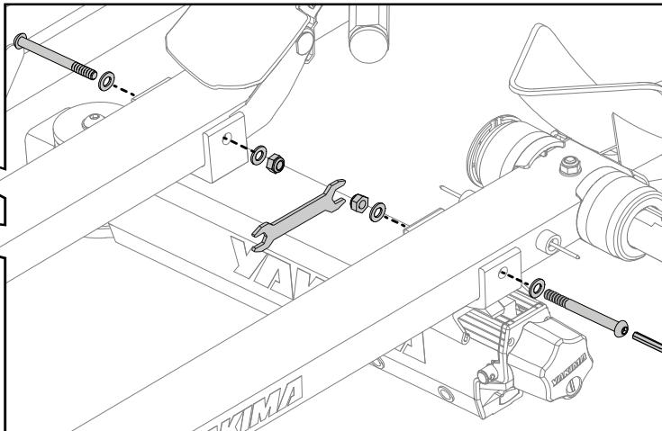
Use the 5 mm hex wrench and a 13 mm box wrench to install the bolts, washers, and nuts as shown. Install the bolts so that the nuts for both wheel tray assemblies face one another between the assemblies.
