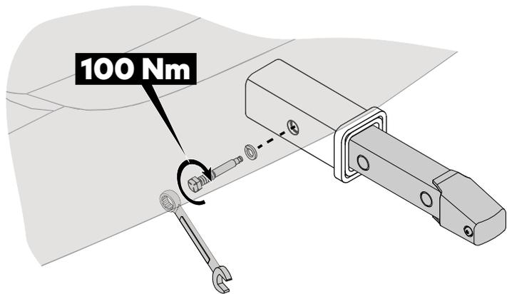
**NOTE:** If there is interference you can install the hitch bolt from the opposite side if you reverse the nut plate. Unscrew the retaining screw, reverse the nutplate, and reinstall the retaining screw. Tighten to 2 Nm.
