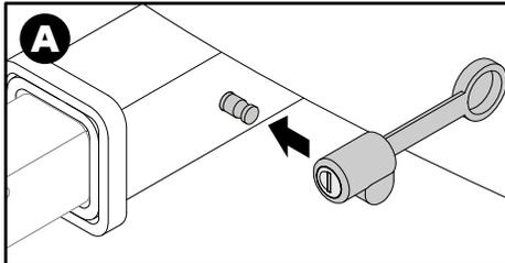
Install the hitch lock and use a key to lock it.
