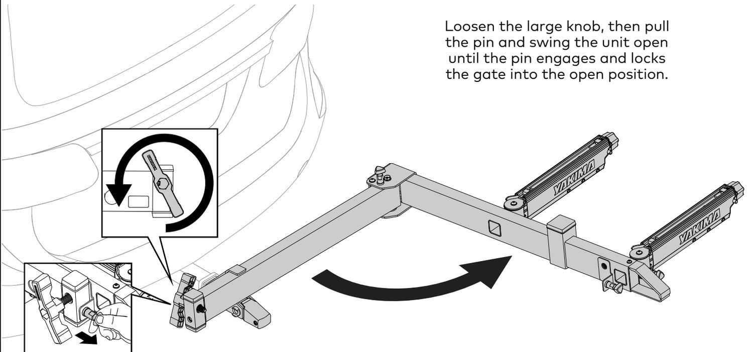
**NOTE:** EXO SwingBase has a 1° upward tilt to prevent sagging while under load.
