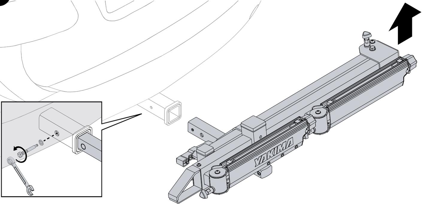
With help from a friend, pull up on the right side so that the EXO SwingBase is level. Use a 24 mm wrench to loosen the bolt, then remove the bolt the rest of the way by hand being careful to not damage the threads of the bolt.
