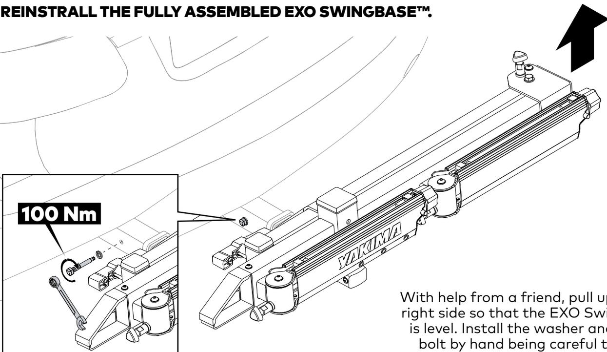
With help from a friend, pull up on the right side so that the EXO SwingBase is level. Install the washer and hitch bolt by hand being careful to not damage the threads of the bolt. Then use a 24 mm wrench to tighten the bolt completely to 100 Nm.
