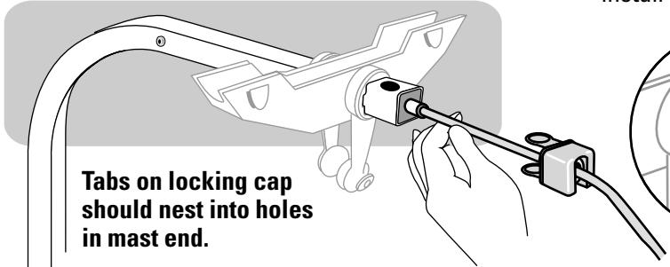
Compress tabs to install locking cap.
