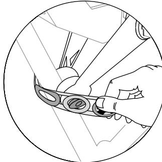
Secure stabilizers by hooking World Straps over bikes tube.
