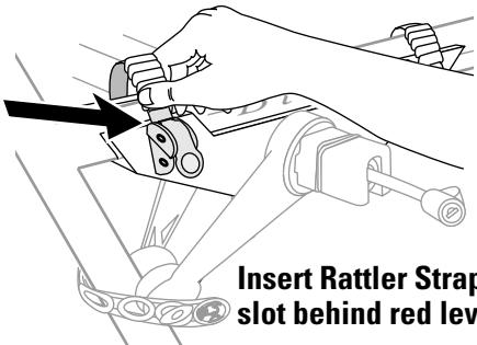
**TO TIGHTEN**, lift red lever up.
