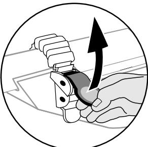
**TO RELEASE**, push red lever and pull up on strap.
