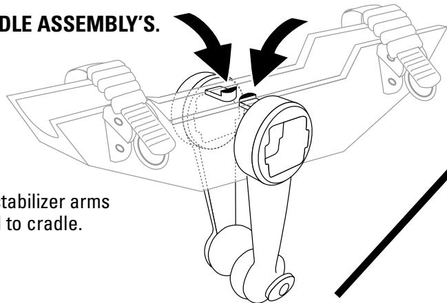
Push cradle assembly onto mast and over stop-button, by
