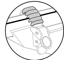
Cables should be routed through slots on underside of strap pads.
