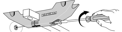
Insert screw and washer into rounded depression on underside of cradle.
