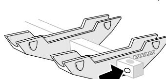
The last cradle must be behind metal rivet.
