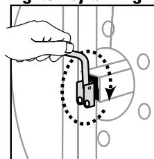
In some models, to fold crank completely, you may need to align crank with a hole or gap in the rim.
