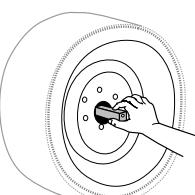
**NOTE:** It may help to hold TreadPlate in place while tightening lug nuts so TreadPlate does not come in contact with rim.
