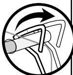
Slide the pin out while supporting the mast.
