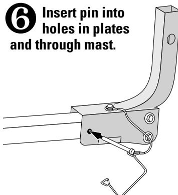
**7** Secure wire onto end of hitch pin.
