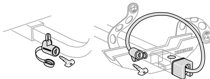
Locking system, locks bikes to mount and mount to receiver.
