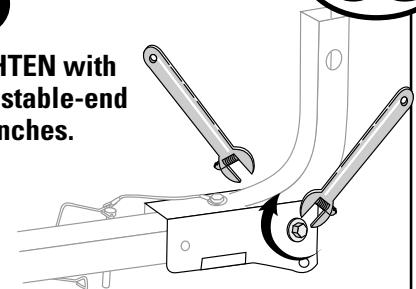
**4** Insert second bolt with a washer into adjacent hole.
