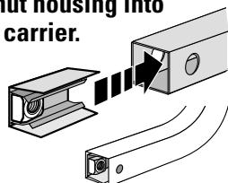
The hole in hitch must align to hole in carrier base.
