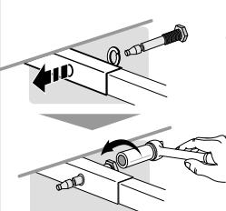
Use a 7/8 or 15/16 inch socket wrench and TIGHTEN.
