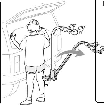
**Don't forget to replace pin AND secure safety hook.**
