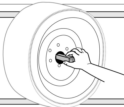
**Some applications may require that you hold TreadPlate in place while tightening lug nuts so it does not come in contact with rim.**
