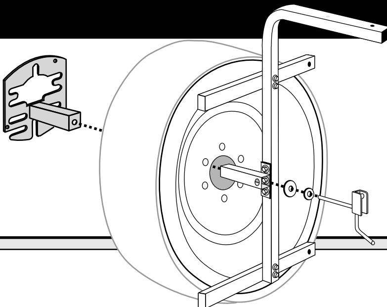
**2 Hang TreadPlate on tire mounting bolts or spare hanger.**
