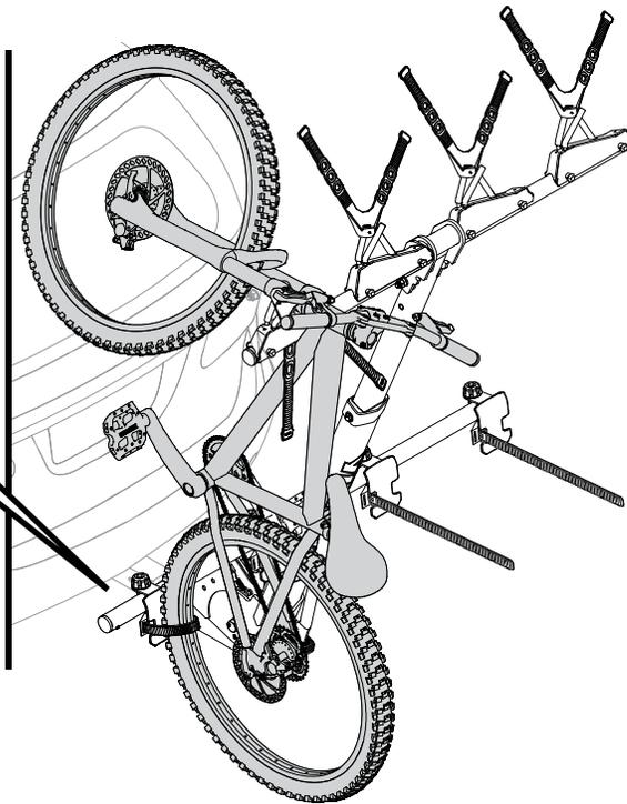
B. For **single crown forks**: secure the front fork with the rubber strap by pulling it **TIGHT** over the fork crown, and securing it to the posts on the cradle by pulling directly out and down over the crown. Secure the right side of the strap first then the left. **NOTE:** Move the lockout lever if it interferes with the cradle.
