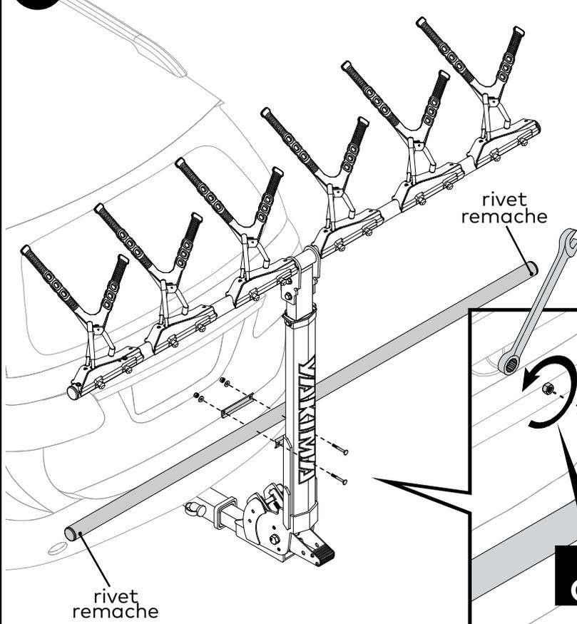
Use the 10 mm wrench to attach the lower bar to the mast with the bolts, plate, washers, and nuts. Make sure that the rivets face outward as shown. Tighten to 5 Nm.
