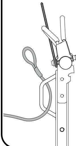
Use the loop on the backside of the mast to route a locking cable.
