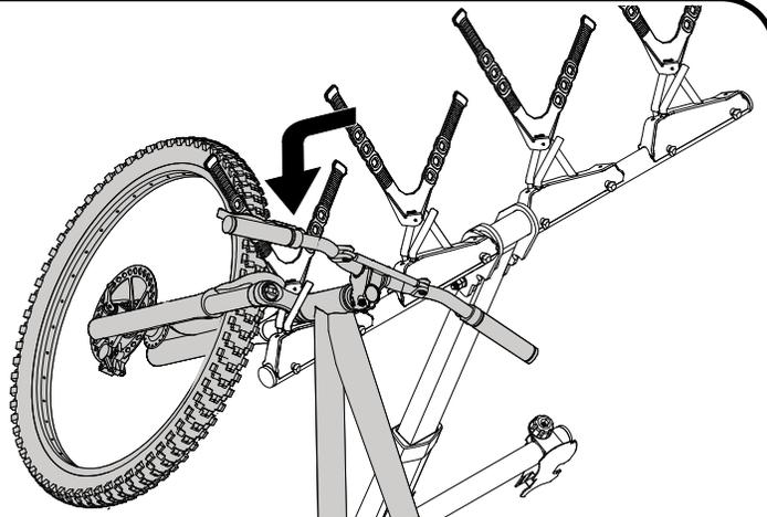
**TIP:** Load the first bike into the left-most spot moving the bike from right to left and setting it into its upper cradle. Then load your other bikes in the same fashion.
