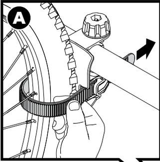
A. Move the rear tire to the wheelcup and secure it with the wheel strap by routing the wheel strap between the spokes and inserting it into the buckle. Pull on the free end to tighten the strap.
