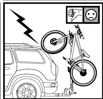
**NOTE:** To increase bike to ground clearance, repeat Assembly step 8.
