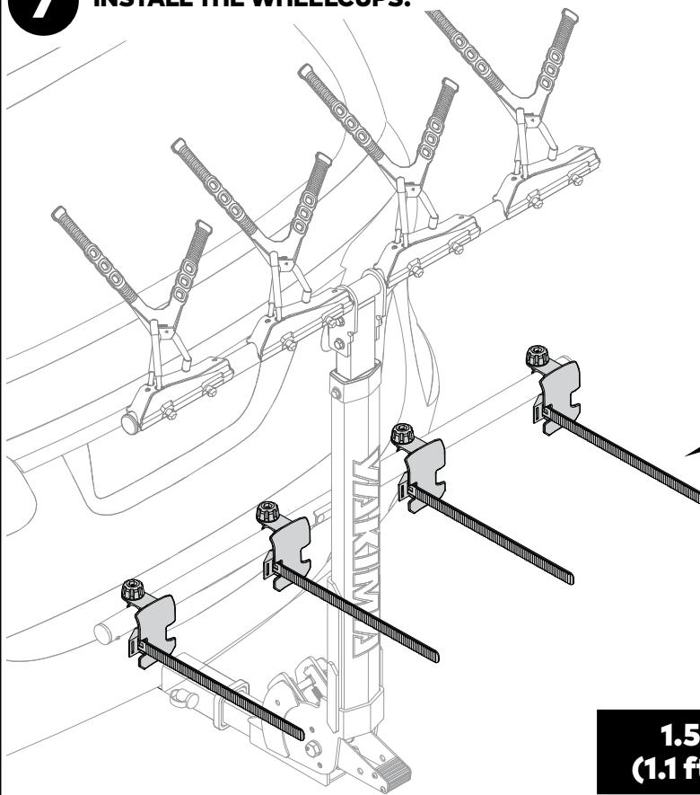
Loosen the knob and flex the wheelcup in order to clear the retention screw on the bar. Then rotate and space the cradles as shown. Tighten the knobs to 1.5 Nm once they are in position.
