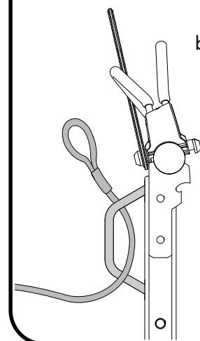
Use the loop on the backside of the mast to route a locking cable.
