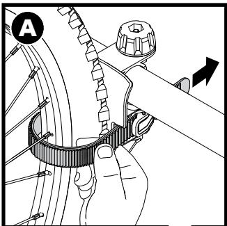
A. Move the rear tire to the wheelcup and secure it with the wheel strap by threading the wheel strap between the spokes and inserting it into the buckle. Pull on the free end to tighten the strap.
