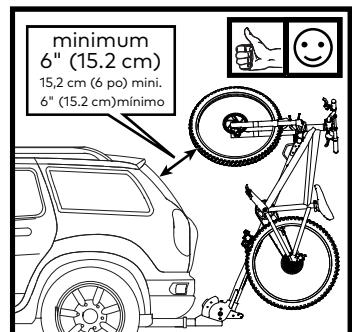
**CAUTION:** Beware of the bike's rear wheel contacting the ground while going over large speed bumps, water bars, steep driveways, and other similar road conditions.
