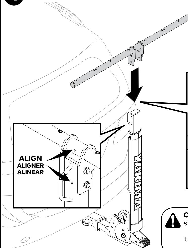
A. Join the top bar to the mast (red dots must be on same side - toward the vehicle). Use the closed wrenches to install the bolts, washers, and hex nuts as shown. Tighten to 15 Nm.
