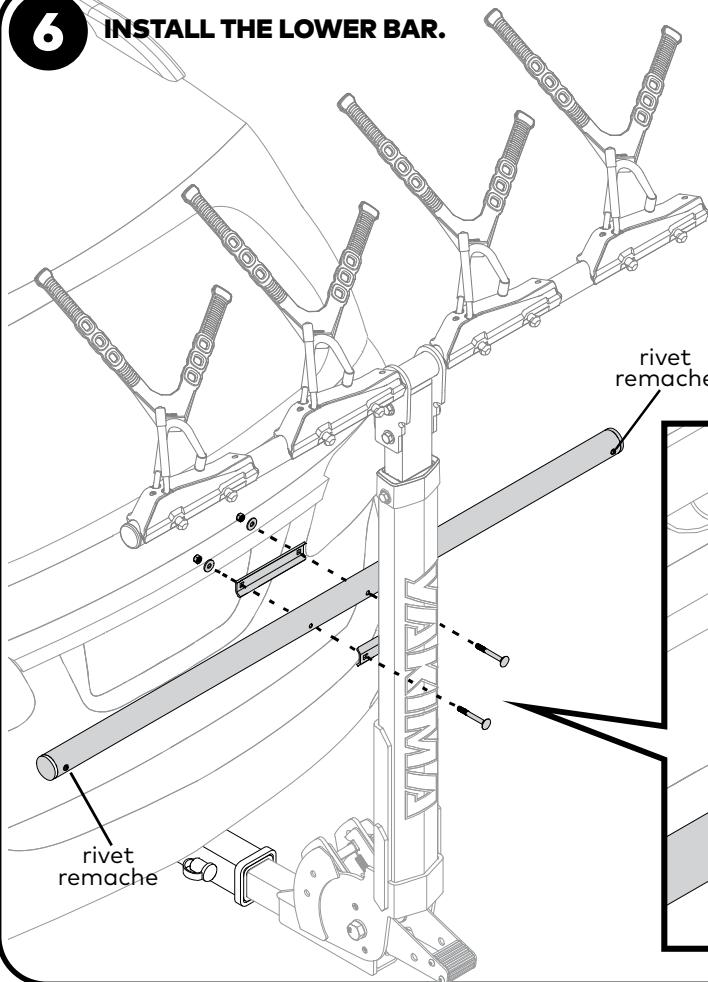
Use the 10 mm wrench to attach the lower bar to the mast with the bolts, plate, washers, and nuts. Make sure that the rivets face outward as shown. Tighten to 5 Nm.
