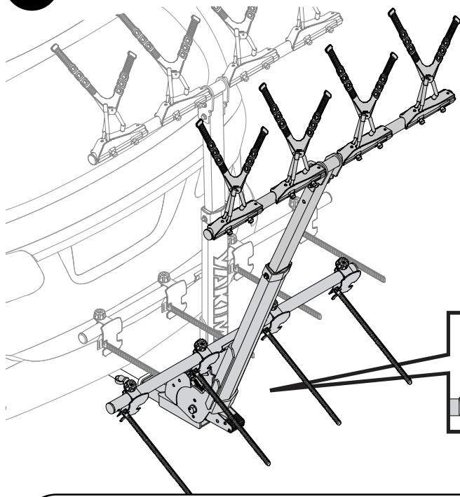
There are two tilt positions to select from. Choose an angle to avoid bike tire contact with your vehicle. The set-back angle works for most vehicles. The vertical position is only recommended for open bed trucks or cars. To adjust the angle, hold the mast with your hand, then step on the foot lever and adjust. An unloaded rack can also be tilted down to access the rear of the vehicle.
