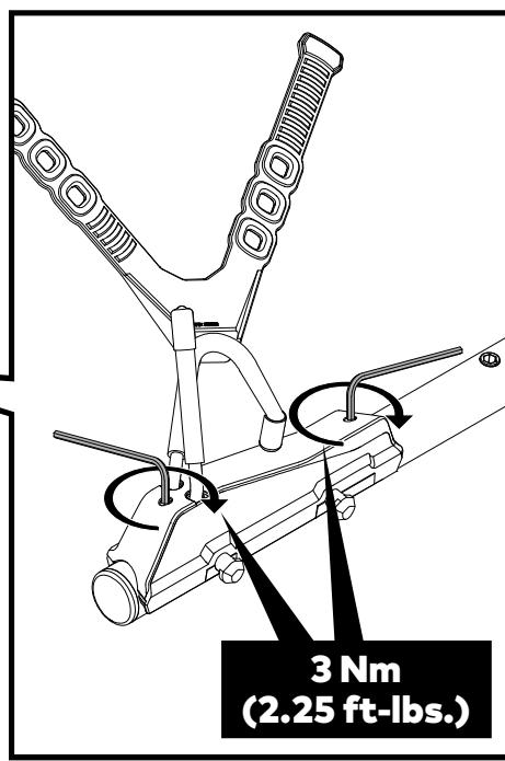
Secure each cradle using the 5 mm wrench. There are two screws built into each cradle. First, loosely install both screws, then tighten each completely to 3 Nm in the order shown.
