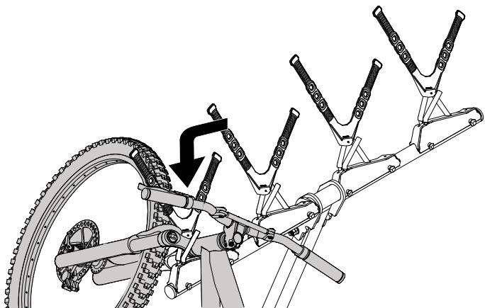
**TIP:** Load the first bike into the left-most spot moving the bike from right to left and setting it into its upper cradle. Then load your other bikes in the same fashion.
