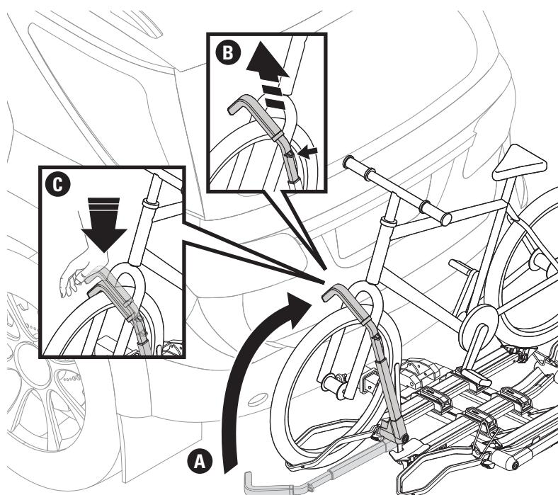
**Failure to place wheel hook in the correct position can cause your bicycle to eject, and cause personal injury, property damage, or death.**
