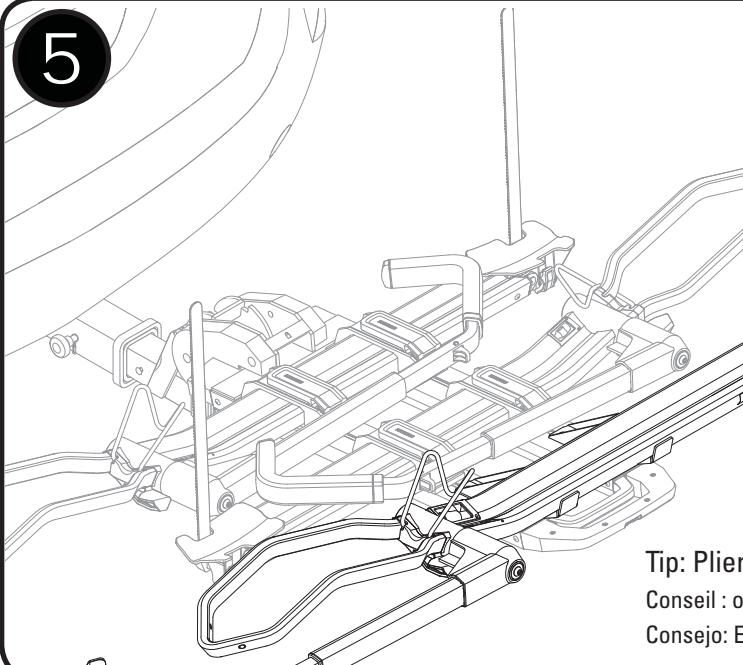
Attach the wheel cup with the lock post. Insert the lock post as shown, and secure it with the e-clip.
