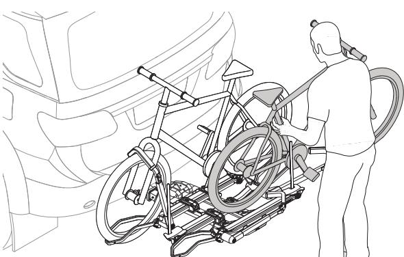
If you have bike to bike interference when loading multiple bikes, adjust trays as necessary to eliminate interference between bikes.
