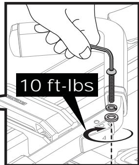
Attach the EZ+1 by installing a washer, lock washer, and screw into each of the 4 holes. Tighten completely.
