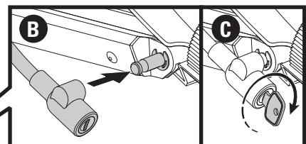
Access locking cables near the pivot arms. Pull the cable out, and pass it through one wheel, around the frame, through the other wheel, and to the lock post. Then lock it. Repeat for your other bike if applicable.
