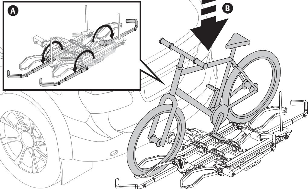
If a fender prevents proper placement of the wheel hook, remove the fender for proper and safe loading.
