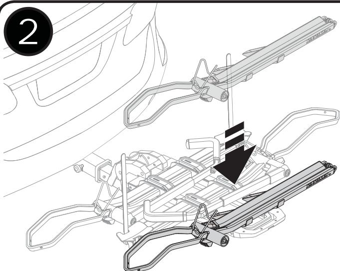
Place the EZ+1 onto Dr.Tray while aligning the four holes.
