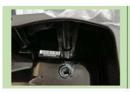
At the bottom of the mast where the large bolt tightens the base to the upright
