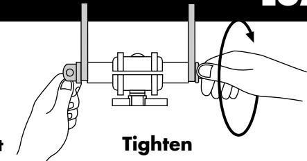
Then close the skewer by flipping the lever 180°. At about halfway through closing you should start to feel resistance. Take care not to over-tighten the lever, but be sure the forks fit snuggly on the skewer. Closing the skewer should take firm pressure—enough to leave an impression on your palm. If the skewer is too loose or tight, open the skewer and adjust it by turning the nut, not the skewer lever.
