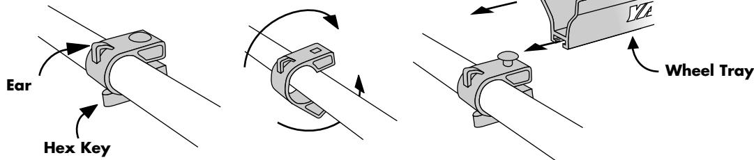
and Hex Key loosely. Slide the Wheel Tray over the bolt head and ear. Tighten the Hex Key.
