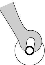
Make sure the front drop-outs are completely down on the ends of the skewer. (If you have difficulty removing your bike forks from the Skewer, throw open the Skewer Lever and loosen the Skewer Nut.)
