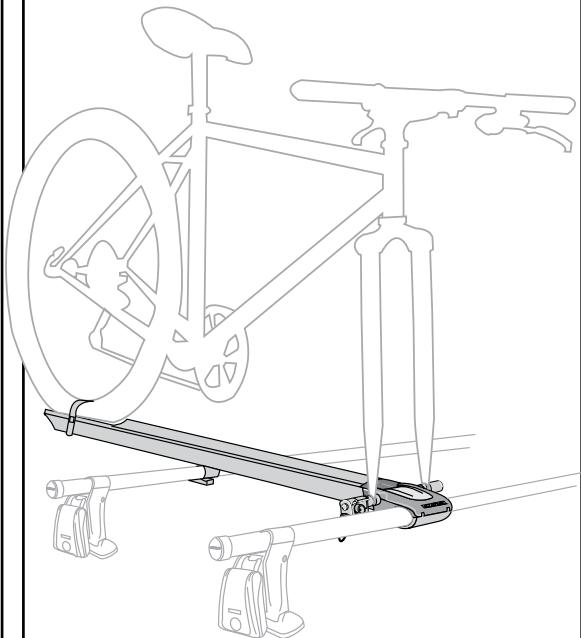
The SteelHead Bicycle Mount secures your bicycle when locked. One SKS® Lock is needed. The mount is secured to your racks by the same lock whether or not a bicycle is loaded.
