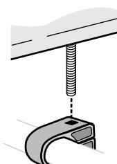
Bolt threads go into square hole in SnapAround. Secure with Hex Key (nut).
