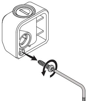
To lock your system, first use the T-15 wrench to remove the screw from each lock housing that came with your OutPost HD™ or OverHaul HD™. Then place the lock housing over the locking post and use a key to lock it.
