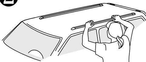
Place both tracks on the roof. Carefully select their locations, making sure they are aligned with each other and symmetrical on the vehicle. Carefully hold the tracks in place with masking tape.
