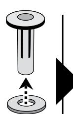
Attach Plusnut® and washer to tool as shown.
