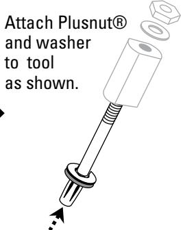
Attach nut with washer onto Plusnut® tool.
