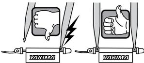
**6** With lever open, tighten nut until the lever closes with some resistance.
