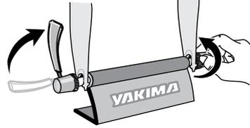
Loosen or tighten the nut as needed so that lever closes with some resistance.
