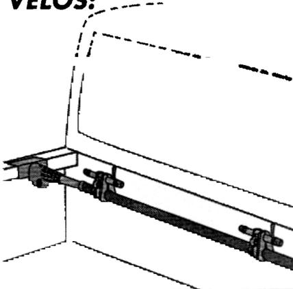
**17** Remove front wheel on bike and set forks onto skewer straight up and down.
