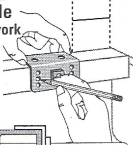
Bracket should rest against the top edge of bed when possible.
