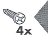
Use this for trucks with bed liners OR where back side of metal is inaccessible. Requires 3/16" drill bit.
