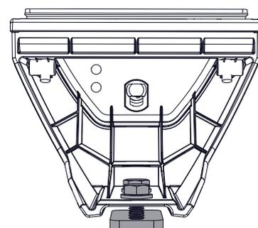
**5** Assemble 1 x M8 Spring Washer and 1 x M8 Washer onto each M8 Hex Bolt in the order shown.
