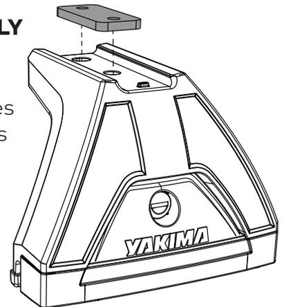
**6** Loosely finger tighten Nut Plates to Legs as shown using the screw assemblies from the previous step.
