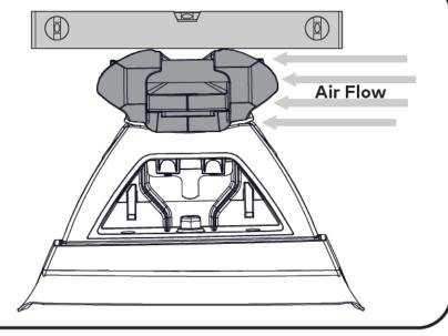
Tighten all M8 Set Screws to 9 Nm using a 13 mm Spanner.
