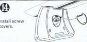
**NOTE:** To remove screw covers, push from inside front of tower.
