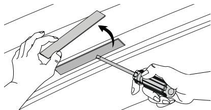
Use a screwdriver to pry up and remove the covers from your vehicle.
