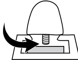
In some cases, it may be easier to assemble plates, screws, and bases before sliding onto tracks.
