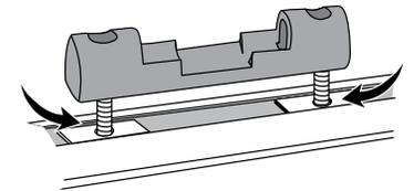
**NOTE:** If screws seem too short and are not engaging the plate, take out screw, remove plastic spacer, use washer only.
