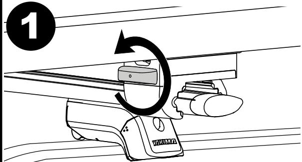
Unlock and open the clamps completely.
