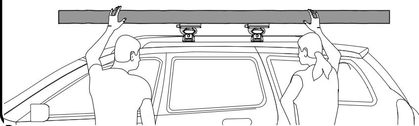
Check for any front to back movement. If there is any movement, repeat step 2 and 4.
