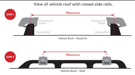
**Attaching directly to SkyLine Tower** STEP 1 STEP 2 STEP 3 Measure: center of Measure: center of Select Landing Pad (L) front roof rack tower Platform to Center of to center of back Size Landing Pad (R) tower Min Max Min Max Size 30" 41.25" 27" 33" К 35.5 46.5" 27" 39" в 46.5" 57.5" 28" 54.5" 1 33.5" 46.5" 28" 54.5" С 30" 41.25" 35" 62.5" Е 35.5" 46.5" 35" 62.5" Ν
