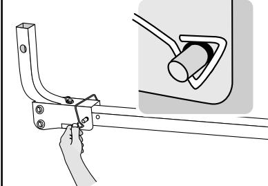
**8** INSTALL HITCH NUT — ATTACH BASE TO HITCH.
