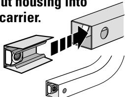
The hole in hitch must align to hole in carrier base.
