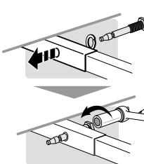
Use a 7/8 or 15/16 inch socket wrench and TIGHTEN.
