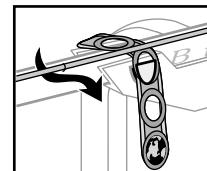
Be sure straps are secured onto cradle hooks.
