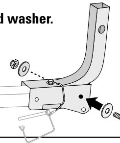
**4** Insert second bolt with a washer into adjacent hole.
