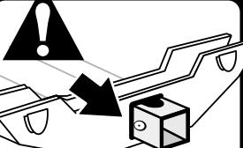
The last cradle must be behind metal rivet.
