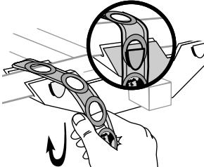
Straps can be routed between cables and tube.
