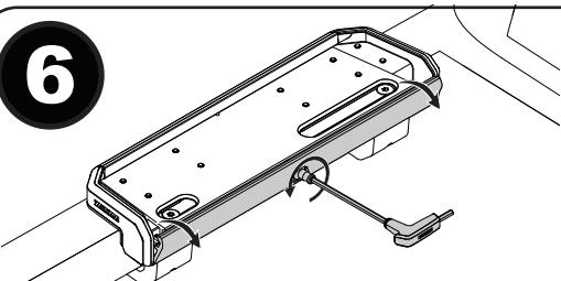
**Open the bases.** Use the 4 mm and 6 mm hex wrenches to loosen the spring loaded receivers.
