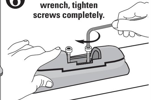
**!** Make sure bases, pads and spacers (if applicable) are fitting tightly into track.
