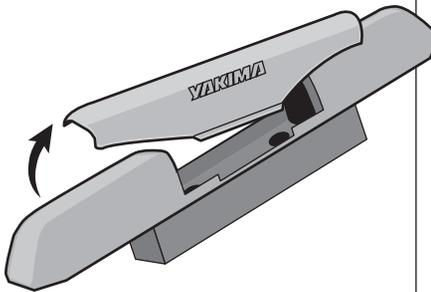
When the racks are not installed, use the covers to keep the bases free of debris.
