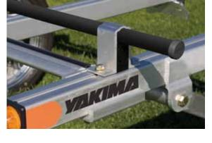
Position Block with Crossbar on top. Slip Tower over T-Bolts. Attach washers and nuts.
