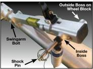
If the Shock Pin does not go in easily, do not hammer it in. Note the black Shock Pin Alignment Screw on the Swingarm (picture 7B). If necessary, adjust screw so when Wheel Block hits it, the Shock Pin holes are lined up for it to go in easily. If the screw sticks out too far, it will prevent the Shock Pin from going in without damage. Please confirm Shock Pin Alignment Screw settings and adjust if necessary.
