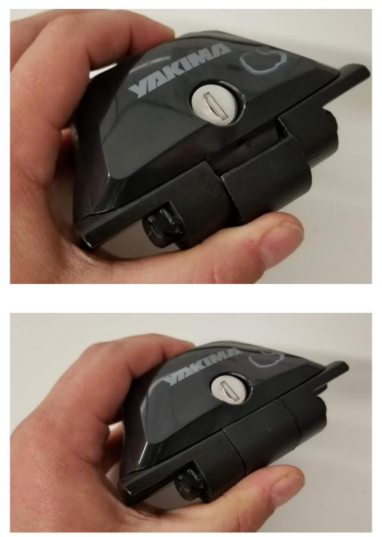
Step 7 – Open and close the door of the tower to ensure proper function. The clip should stay in place with no gaps and the tabs should push outward when the door is closed and retract inward when the door is open.
