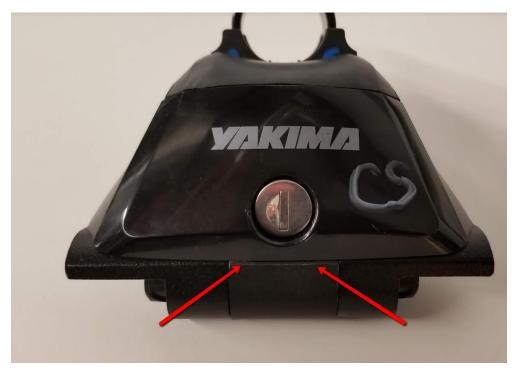
**Step 2** – Remove the clip by continuing to pull downward from the tower. It should release fairly easily.
