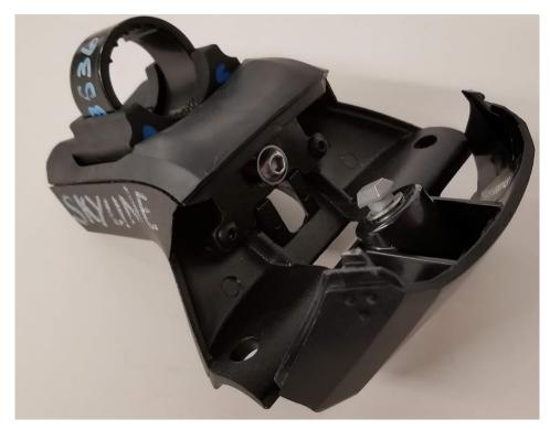
**Step 4** – Pull straight out on the door. It will release from the little retractable tabs in the tower. Be sure not to move those tabs and ensure they remain lined up on the same plain.
