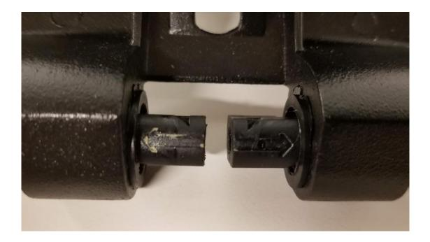
**Step 5** – Install new door by pressing the door over the tabs. Simply the reverse of how you took the door off.
