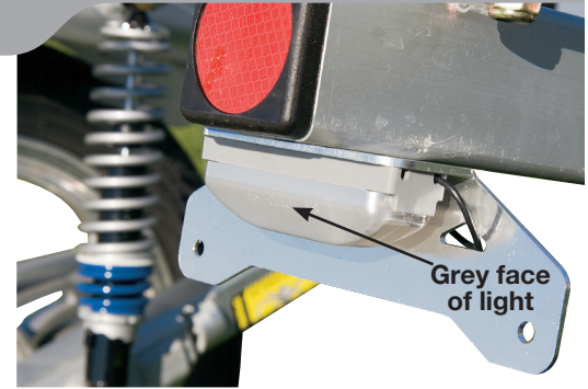
License Bracket & Light installed
