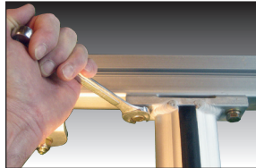
6C Tighten 16 bolts to 31 ft. lbs. (42N-m)
