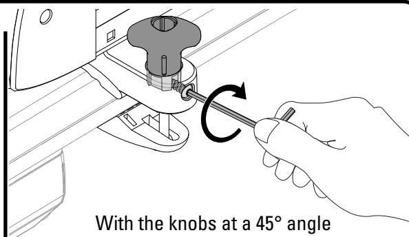
With the knobs at a 45° angle use the security wrench to tighten the security screws. Check that the knob doesn't turn.
