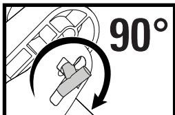
Close the mounts. Rotate the t-bolt and open the clamps. Then place the mounts onto the crossbar.
