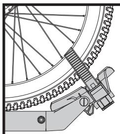
**IMPORTANT:** For bikes with 20" wheels, if the wheelbase is less than 35", the rear wheel may not contact the wheel cup. Ensure that the wheel strap is pulled tightly, and secured in the buckle (see image). Also tires must be fully inflated, and centered on the tray.
