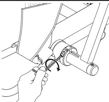
Periodically it may be necessary to adjust the tension of the pivot arm. Use the security wrench to make the adjustment.
