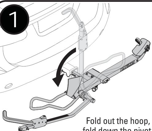
Fold out the hoop, and fold down the pivot arm.
