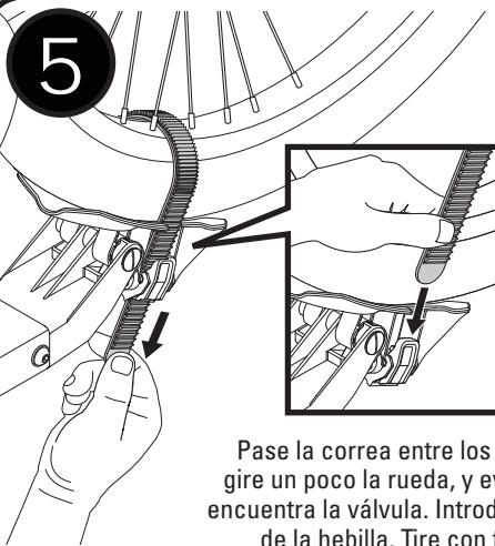
Feed the strap through the spokes of the wheel. Rotate the wheel slightly, if necessary, and avoid the valve stem. Insert the strap end through the buckle. Pull hard to tighten.
