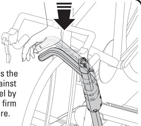
Compress the hook against the wheel by applying firm pressure.
